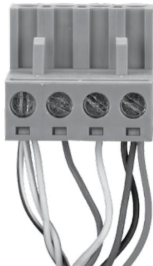
1. Ground connection (GND) -> connect to RJ45 pin 1 and 3 and 7 (colours : see table below)
