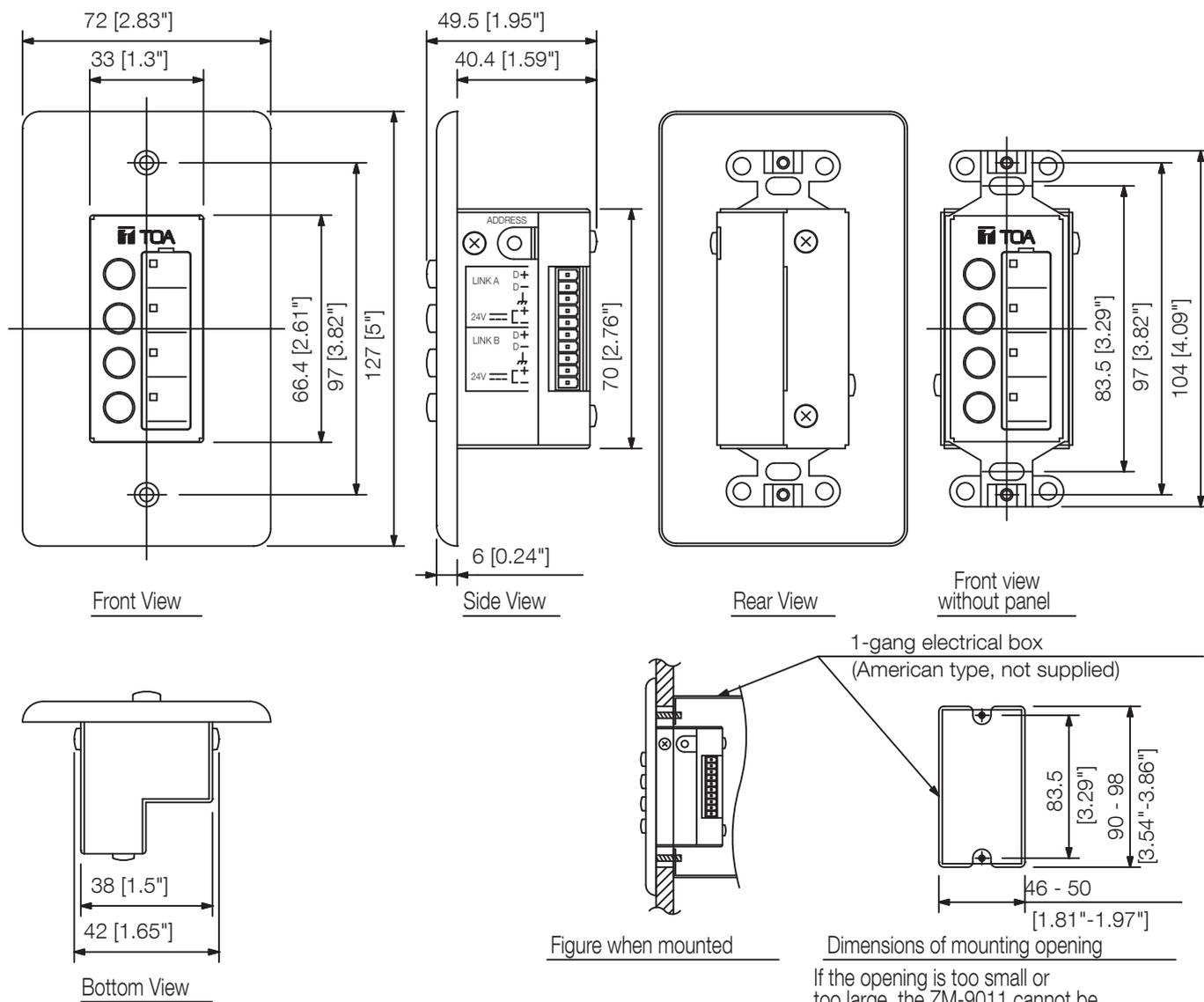
If the opening is too small or too large, the ZM-9011 cannot be mounted in the wall. Be sure to make an opening with dimensions given above when mounting.
