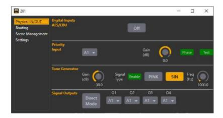
Set analogue and digital input and output configuration.
