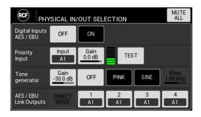
**Digital Inputs AES/EBU** — Enable / disable 4 digital inputs AES/EBU (D1 - D2 - D3 e D4) alternative to analogue inputs A3 and A4. These inputs are physically allocated on two connectors.
