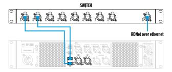
Each XPS 16K device must be connected to a different switch port.
