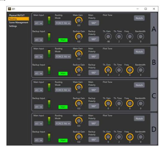
Set, for each output, main and backup inputs parameters, and routing strategy.
