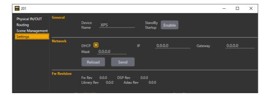
Set general (e.g. device name) and network configuration parameters.
