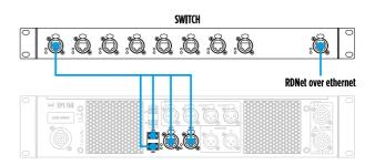
Connecting 2 different ports of the device to the external switch a full redundancy is achieved.
