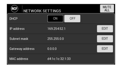
**DHCP** – set Dynamic Host Configuration Protocol ON or OFF. If set ON, the following parameters IP address, Subnet mask and Gateway address are assigned automatically and not editable.
