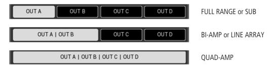
Changing the **SPEAKER MODEL** setting, all outputs and routing parameters will be consequently reset. A confirmation popup will ask user to confirm the action.
