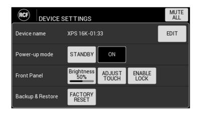
**Device name** – set a custom name for the device, to better identify it in a system.
