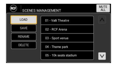
It shows the list of the scenes saved on the device. The toggle buttons on the left side of the screen provide the related function.
