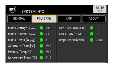
Shows the status of device power supply and fans operativity parameters.
