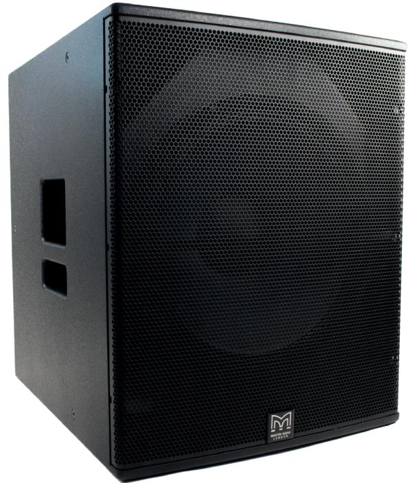
The X118 is a compact, high performance subwoofer for use with BlacklineX Series full-range loudspeakers. It extends the low frequency operating range of the combined system to 42Hz and provides exceptional low frequency impact. It can be used singly, stacked or flown via integral M10 insets and features a long-excursion 18" (460mm)/3" (75 mm) voice coil driver in a compact reflex enclosure. Its four reflex ports have a large frontal area to reduce turbulent air noise at very high levels.
