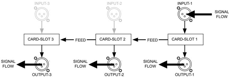
The FEED switch allows you to daisy chain a series of adjacent modules making it easy to create a customized channel strip whereby a mic preamp feeds an EQ which in turn could feed a compressor. Changing the order is simply a matter of relocating the modules or patching using an XLR cable. The UP position turns the FEED connection on.
