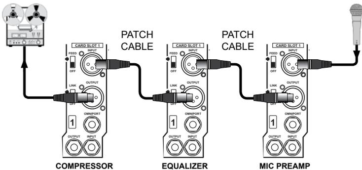
The Cube simplifies the process with a FEED switch that replaces inter-module patch cables. Instead of using an XLR cable, you simply push the FEED switch into the UP position and it routes the signal to the adjoining module's input. When engaged, the FEED function sends the signal to the next module working from left to right (front view). Because the FEED function is tied to the XLR connector, it will work with new Radial modules and older 500 series modules.
