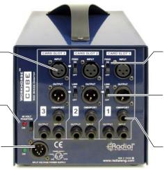
FEED SWITCH: Sends the output from one module into the next without requiring a cable.
