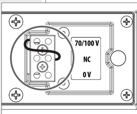
The two terminals ('70/100V' and '0V') allow to connect both input and output cables (to link other speakers in parallel).
