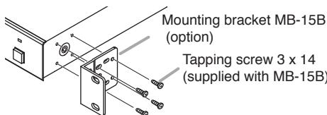
**Step 2.** Using other screws also supplied with the MB-15B, mount the unit in the rack.
