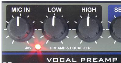
Microphone preamp with two band EQ and phantom power for condenser mic.
