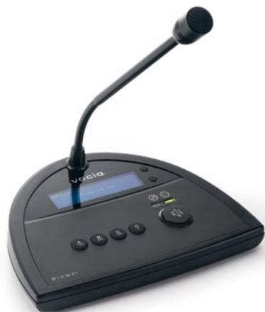
The DS-4 is a desktop networked paging station featuring embedded DSP, on-board memory, and PoE supporting both standard and advanced public address functionality. All device-specific configuration information is stored locally, which means the DS-4 does not rely on a centralized controller for processing and page routing.
