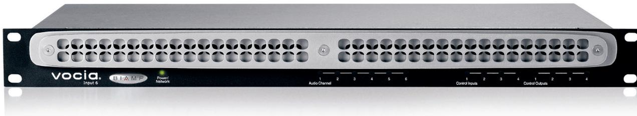
The VI-6 is a networked audio input expansion device allowing the user to add up to six channels of audio to a Vocia system. It supports up to six background music inputs, six individual user-configurable paging inputs or four dedicated paging inputs using the Vocia Auxiliary Microphone (VAM-1). The VI-6 features embedded DSP and on-board memory to process and store all device-specific configuration information locally and includes comprehensive, fixed-chain DSP.
