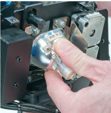
Replace the lamp by setting the lamp into the two bottom brackets, gently press the lamp down, and insert the top of the lamp into the lamp frame.
