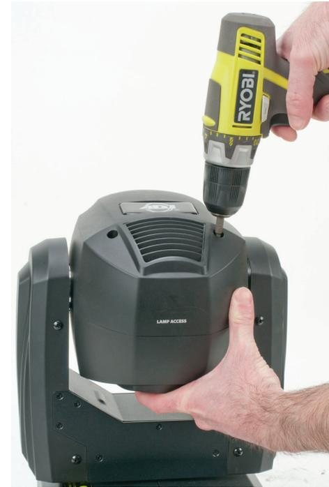
Replacing the lamp is relatively easy. Unplug the unit from its power source. Allow the unit 15 minutes to cool down. Remove the shell that says “Lamp Access” on the rear. Start by unscrewing the four phillips screws that hold the shell in place. Once the screws are unscrewed remove the shell. You will now have access to the lamp.
