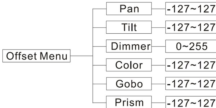
To enter the Offset Menu, press the ENTER button for at least 5 seconds. In this submenu you are able to adjust the home position of the pan, tilt, shutter, color wheel, gobo, and prism.
