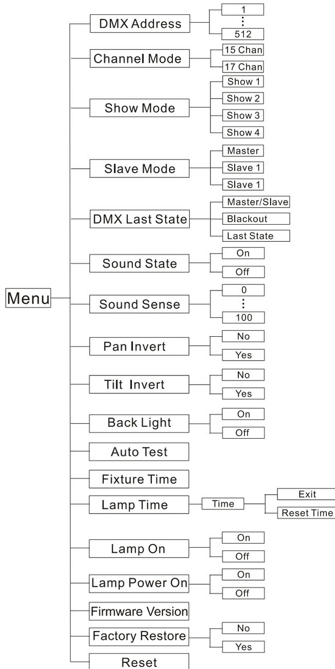
**System Menu:** When making adjustments press **ENTER** to confirm your setup then press and hold the **MENU** button for at least 3 seconds. To exit without making any adjustments press the **MENU** button. The display will lock after 30 seconds, press the **MENU** button for 3 seconds to unlock.
