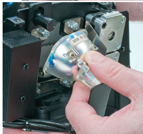
**Fixture Cleaning:** Due to fog residue, smoke, and dust cleaning the internal and external optical lenses and mirror should be carried out periodically to optimize light output. Cleaning frequency depends on the environment in which the fixture operates (i.e. smoke, fog residue, dust, dew). In heavy club use we recommend cleaning on a monthly basis. Periodic cleaning will ensure longevity, and crisp output.
