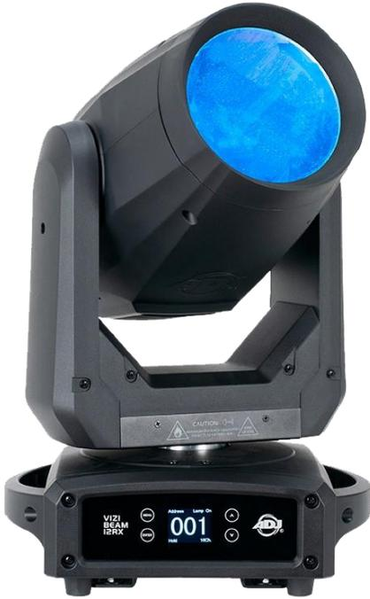
The Vizi Beam 12RX is high powered beam moving head powered by the brilliant 260W Philips® Platinum 12R LL MSD Discharge Lamp (6,000 hr.). It produces a razor sharp 2-degree beam of light. It comes with 14 colors + open (with color indexing), 16 fixed GOBOS + open, two rotating prisms and a frost filter for wash effects.
