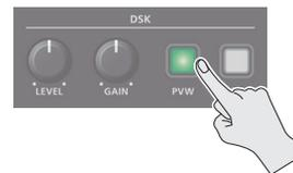
The DSK [PVW] button lights up in green, and a preview of the composition results is displayed in the PVW section of the monitor.
