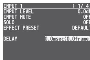
3. Turn the [VALUE] knob to adjust the time by which the audio is delayed, and press the [VALUE] knob.
