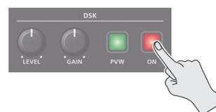
The DSK [ON] button lights up in red, and the composition results is sent to final output.
