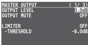
6. Turn the [VALUE] knob to adjust the output volume, and press the [VALUE] knob.
