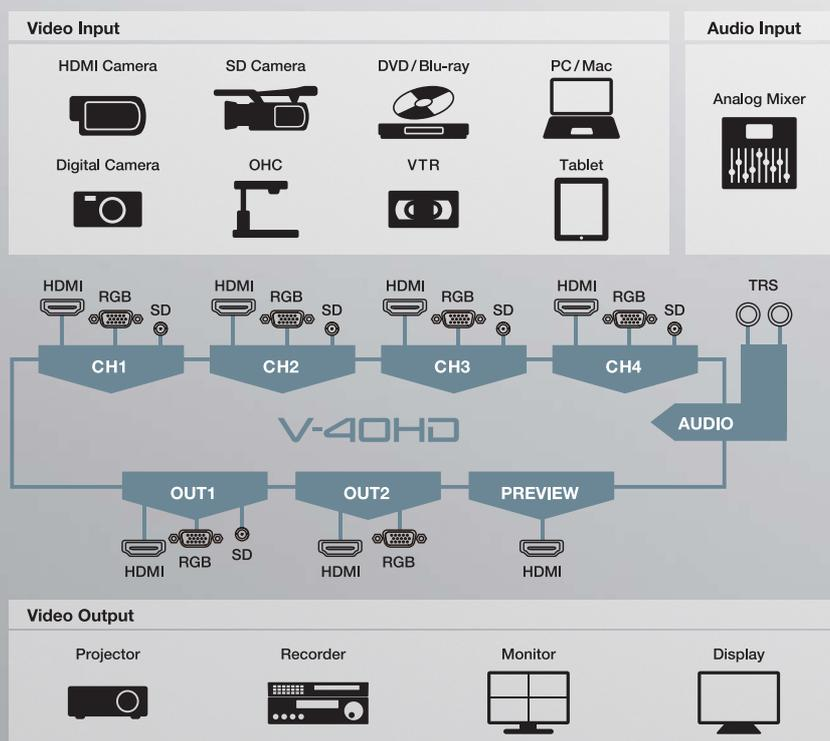
\*RGB connectors support RGB or component signals.
