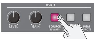
2. Press a DSK SOURCE [1]–[10] button to select the DSK video source.
