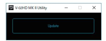
"V-02HD MK II Utility" is dedicated software for the V-02HD MK II. It lets you connect the V-02HD MK II to your computer via USB, and backup/restore the settings of the V-02HD MK II unit, or update its system program.
