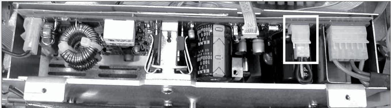
In the picture 1, the voltage change connector is highlighted by a square.
