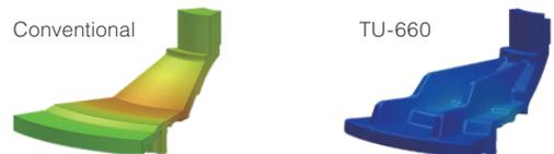
In the TU-660 we added a heat-dissipating fan at the upper cover and increased the surface area, and these two measures combined have doubled heat dissipation.
