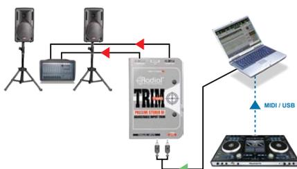
**Using the Trim-Two in a keyboard setup**
