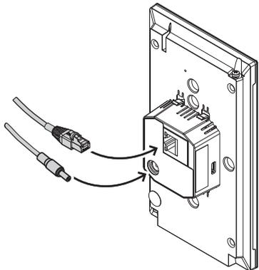
PoE connection requires IEEE 802.3af standard. Use a network switch or PoE injector that meets this standard. Connect the device using a standard T568A or T568B Ethernet cable.
