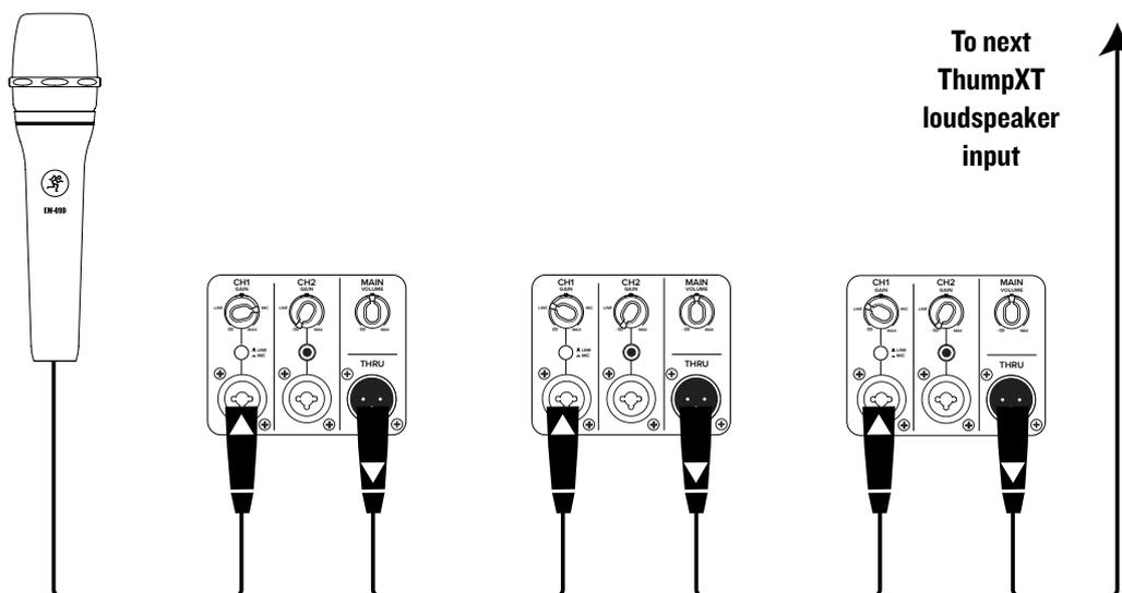
ThumpXT loudspeakers may be daisy-chained via the “THRU” jack which outputs all inputs. Simply plug the signal source (i.e., mixer output or microphone) into the input jack(s), and patch that loudspeaker’s mix out jack to the next loudspeaker’s input jack, and so on, daisy-chaining multiple ThumpXT loudspeakers. See above for visual representations of daisy-chaining.
