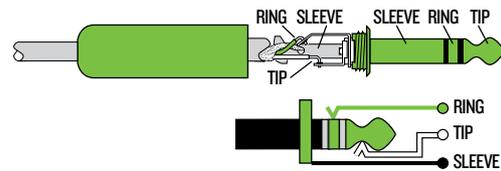
To connect unbalanced lines to these inputs, use a 1/4" mono (TS) phone plug, wired as follows:
