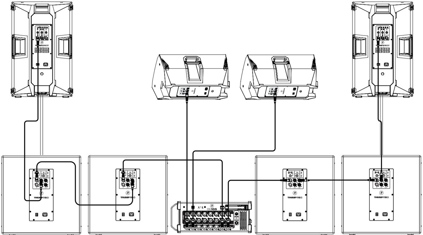
Here's how to set up a large club system. In this example, the L/R outputs of a DL16S mixer are connected directly to the channel A inputs of a pair of Thump118S subwoofers. The Full Range Out of each subwoofer is then connected to the inputs of an additional pair of Thump118S subwoofers.
