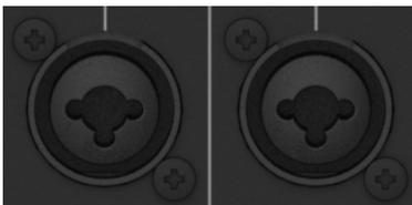
Input channels 1 and 2 may accept a balanced mic signal using an XLR connector.
