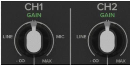
If you haven't already, please read the "Quick Start" section on page 6. Setting the gain correctly will ensure that the preamplifier's gain is not too high, where distortion could occur, and not too low, where the quieter, exquisitely-delicate passages might be lost in background noise.
