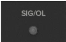
This dual-colored LED will illuminate green when the input signal is present, indicating signal.
