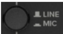
Because an XLR connector may be connected to a mic or an instrument, this switch adjusts the channel's input sensitivity to optimize channel 1 for mic or line-level signals. If a mic is connected, this switch should be engaged and the gain knob set to mic. If an instrument is connected to channel 1 (via XLR), this switch should be disengaged and the gain knob set to line.
