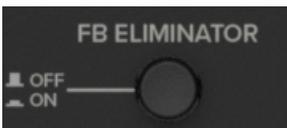
The multi-band feedback eliminator hunts down offending feedback frequencies and applies up to six notch filters automatically to destroy feedback and maximize gain prior to feedback. This is a great tool for when an engineer is not present.
