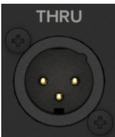
This is a male XLR-type connector that produces the mix from the input jacks. Use it to daisy-chain several Thump loudspeakers together off the same signal source(s).
