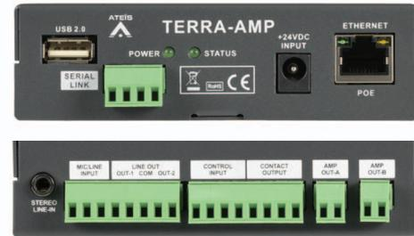
TERRA-AMP is an IP audio terminal with built-in 2 x 15 W amplifier on two independent balanced outputs, USB flash memory interface for playlist backups or prerecorded announcement, 1 mic/line balanced input. In a lot of applications this amplified IP terminal for 8-ohm speakers reduces price and space. The ideal solution for Commercial audio & Public Address systems. The mic & line inputs can be played locally or can be used as a source for a network stream.
