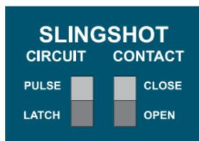
Just imagine... being able to switch amps while activating a rackmount digital delay or in-amp spring reverb. Slingshot™ is a contact closure system that works with all kinds of devices to let you perform various tasks using a single foot-stomp. Add devices such as the Headbone™ head switcher or Cabbone™ cabinet switcher to change channels, heads
