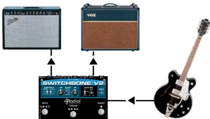
You will note that when you hit the BOTH footswitch, one of the LEDs will begin to flash. This TOGGLE mode function is designed to let you know in advance what will happen when you hit the BOTH footswitch again whereby the flashing LED will be the one that goes off. You can toggle the flashing LED by depressing the AB selector footswitch so that when you return to single amp playing, you can ensure the amp that you want on will be the one that is active.
