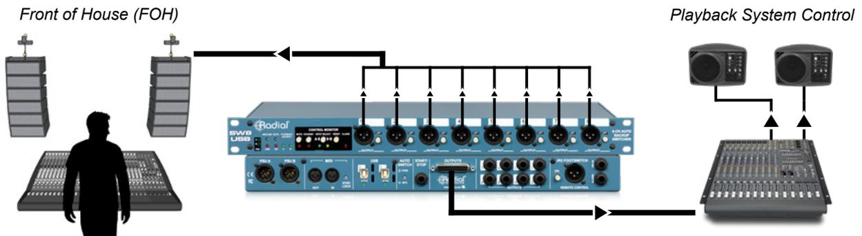
**XLR OUTPUTS:** The front panel XLR outputs feature DI box transformers that provide isolation to eliminate hum and buzz from ground loops when connecting to distant PA systems. Individual ground lift switches are also provided on each channel to further eliminate noise.
