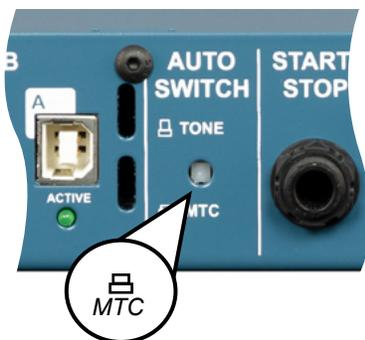
To feed MTC (MIDI Time Code) to the Auto-Switch inputs, set the rear panel AUTO-SWITCH input selector to the 'in' position. Then setup your Digital Audio Workstation (DAW) to feed MTC to the SW8-USB. This will require you to enable the MTC generate/transmit function in your DAW, and to select the SW8-USB as the output destination. Refer to the user guide for your DAW for details on where these settings are located (ProTools MTC settings shown below).
