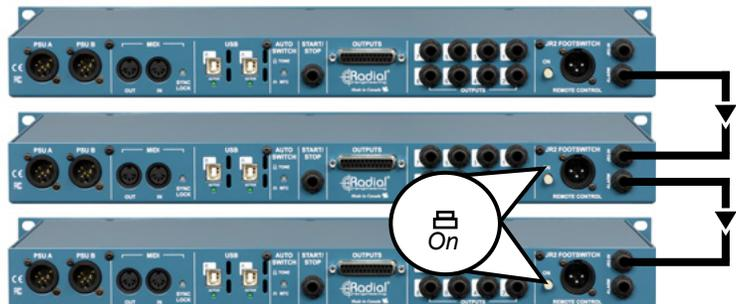
Linking multiple SW8-USB units using 1/4" TRS cables
