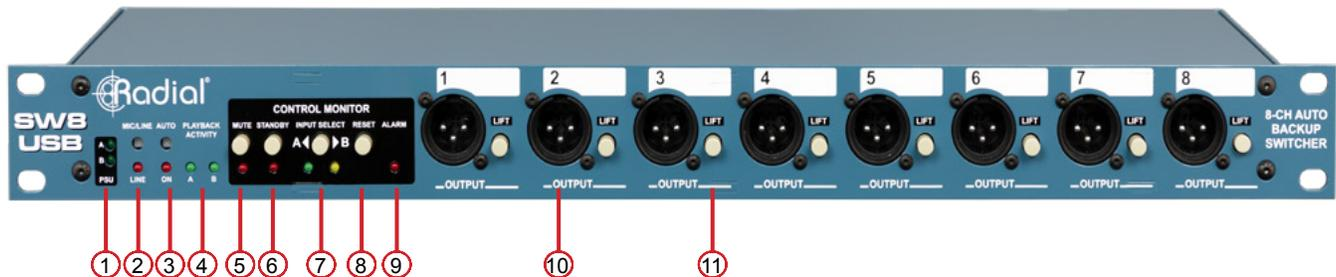
1. **PSU A/B:** Dual LEDs indicate that the SW8-USB is receiving power from each power supply. Only one connection is required to power the SW8-USB, the other is provided for redundancy to eliminate loss of power.
