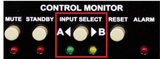
The **INPUT SELECT** switch on the front panel
