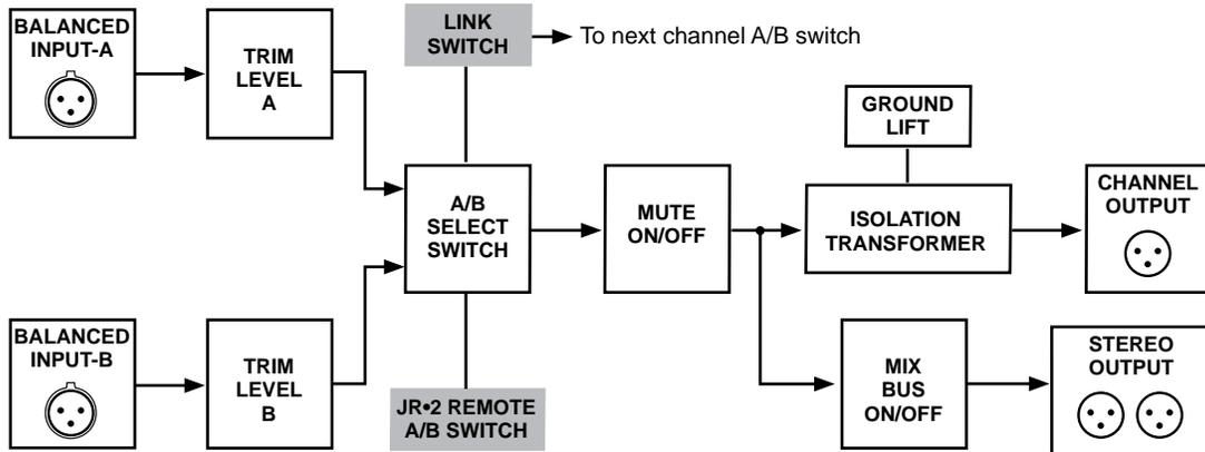
To eliminate hum and buzz caused by ground loops, each channel output is transformer isolated and equipped with a ground lift switch. These are rated to handle signal levels in excess of +20dB from 20Hz to 20kHz and work equally well when switching the outputs from professional mixing consoles as they do for wireless microphones and instrument level signals.
