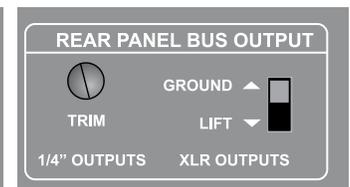
Trim control for the mix bus 1/4" outs and ground lift for the XLR outputs.
