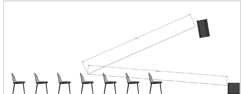
In this example, the Cuboid has been wall-mounted, and Sub is on the floor. Decide on a Recommended Listening Position (RLP), usually halfway through the coverage area. Measure the distance to each speaker.
