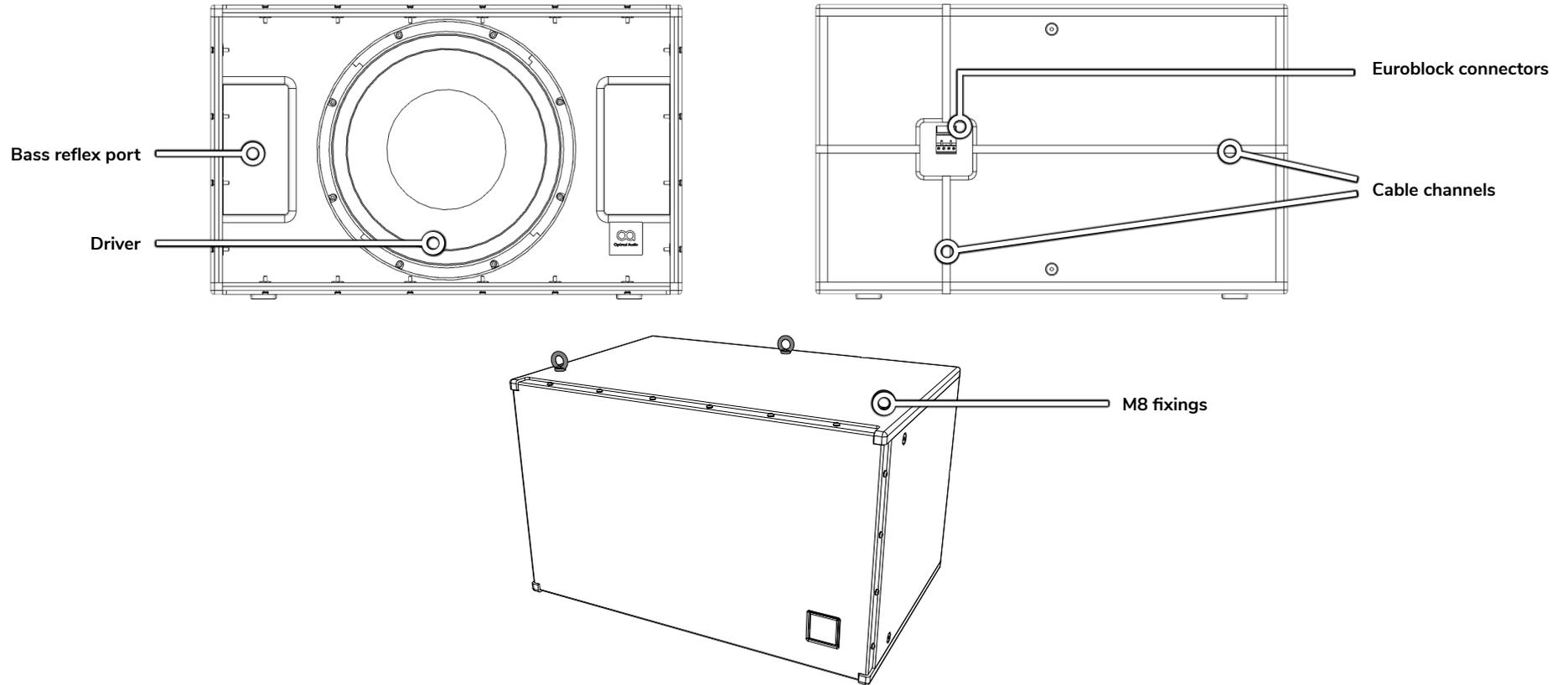
Sub 6, Sub 10 and Sub 15 are passive, low-frequency loudspeakers. Each model consists of a single driver loaded into a compact bass-reflex cabinet.
