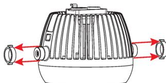
Install the head-only yoke with the yoke knobs
