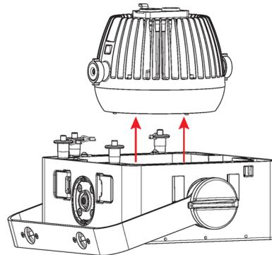
Remove the friction plates
