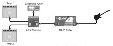
Drive two amps and a tuner through a Radial BigShot AB/Y switcher.
