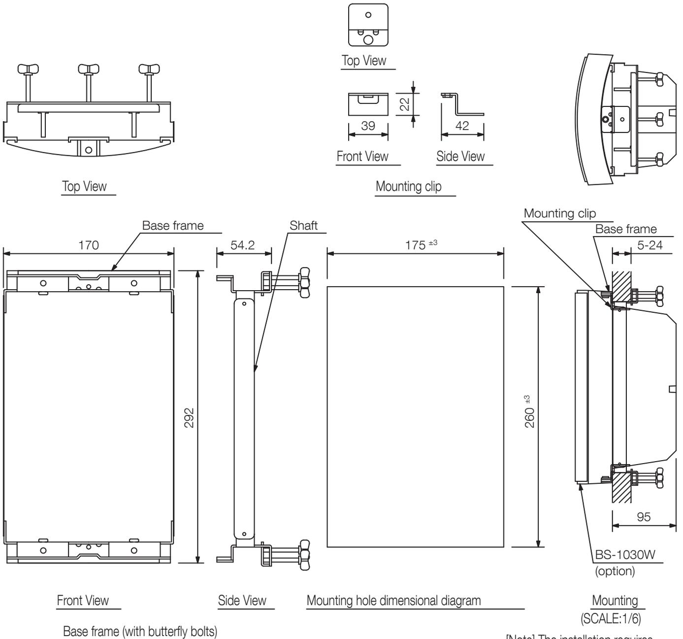
[Note] The installation requires a space of at least 95 mm from the ceiling or wall surface.
