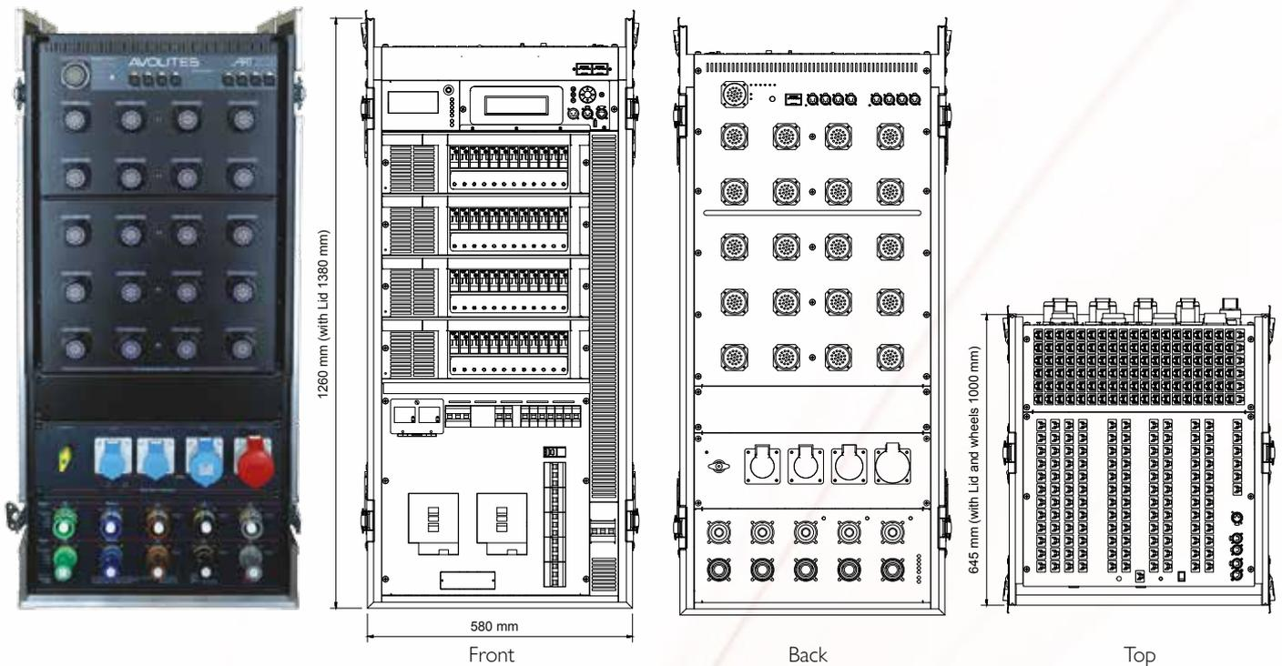
The Dimmer modules have 'load check' indicators for each dimmable channel to give a positive indication that a load is present and the local test fader on each dimmer channel to ensure that you can easily check the connected load without having to use a console.
