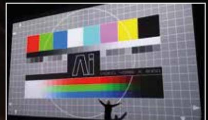
Multiple servers are also supported in the automated warp and blend process using an IP camera. This allows blends across huge surfaces. Curved surfaces, domes and flat screen arrays are all supported. This feature comes as standard with all Ai products and Software Licences.\*
