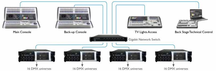
Networking of the outputs using the TNP increases system capabilities to up to 64 DMX universes, catering for even the largest world class spectacles. All of this can be used in conjunction with Titan Remote!
