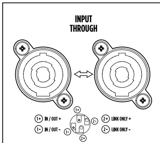
Connect the positive wire (amplifier '+' output) to the pin 'IN / OUT +' of the 4-pin SPEAKON connector. Connect the negative wire (amplifier '-' output) to the pin 'IN / OUT -' of the 4-pin SPEAKON connector. The 'LINK ONLY +' and 'LINK ONLY -' pins are useful to link another subwoofer in parallel.
