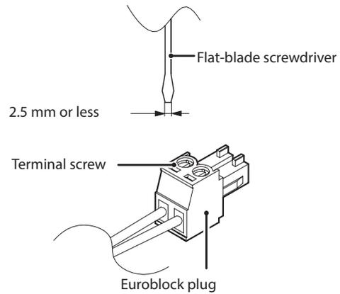
1. Loosen the Euroblock plug terminal screws.
