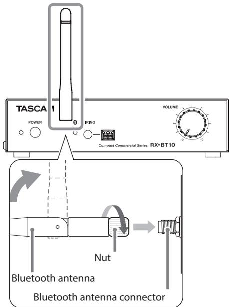
1. Attach the included Bluetooth antenna to the Bluetooth antenna connector.
