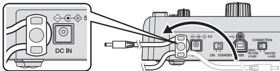
③ Turn the tip of the power cord so that it is facing towards you, then turn it back to create a ring as shown in the diagram and insert it into the [DC IN] terminal of this unit.
