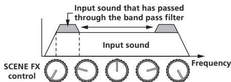
**SCENE FX control** Sets the band pass filter's cutoff frequency.
