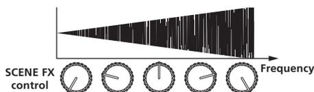
**SCENE FX control** Sets the cutoff frequency of the filter through which the white noise passes.
