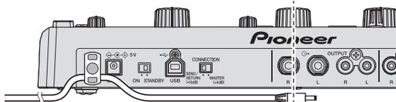
② As shown on the diagram below, move the tip of the power cord back in the opposite direction past the top of the cord hook, and hook the power cord onto the top side of the cord hook.
