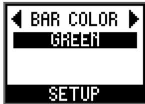
3. Turn the encoder with switch to select OFF (not lit), GREEN (lit), or BLUE (lit), and then press it to confirm.
