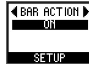
3. Turn the encoder with switch to select OFF (not lit), BLINK, or ON (lit), and then press it to confirm.
