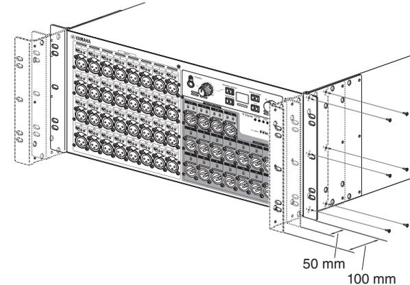
In the same way, rack mount hardware can also be attached to the rear panel surface.
