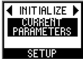
4. When you see the message "CURRENT PARAMETERS INITIALIZE?," turn the encoder with switch to select OK, and then press it to confirm. Initialization of the HA and OUTPUT parameters begins.
