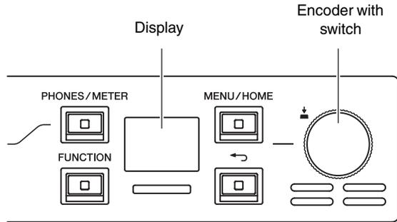
You can use the front panel display, [PHONES/METER] key, [FUNCTION] key, [MENU/HOME] key, [↩] (Back) key, and the encoder with switch to set the various parameters.
