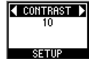
3. Turn the encoder with switch to select a value, and then press it to confirm.
