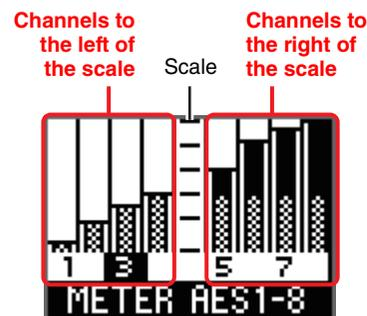
An example of selecting one of the channels to the left of the center scale
