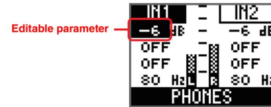
3. Press the encoder with switch repeatedly to highlight the parameter you want to edit, and then turn the encoder to modify the parameter value.
