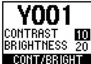
3. While continuing to press and hold the [↔] (Back) key, turn the encoder with switch to modify the parameter value.
