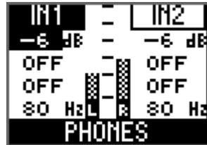
You can set the following parameters for the OUTPUT channel (including AES on the Rio3224-D3) assigned to PHONES.
