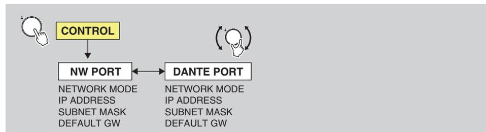
While the CONTROL screen is displayed, turn the encoder with switch to select a parameter, and then press it to confirm.
