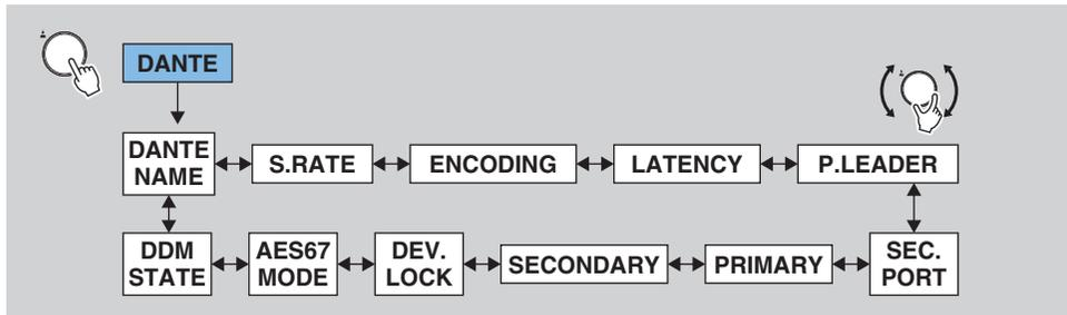
While the DANTE screen is displayed, turn the encoder with switch to select a parameter.
