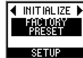
4. When you see the message "FACTORY PRESET INITIALIZE?," turn the encoder with switch to select OK, and then press it to confirm.
