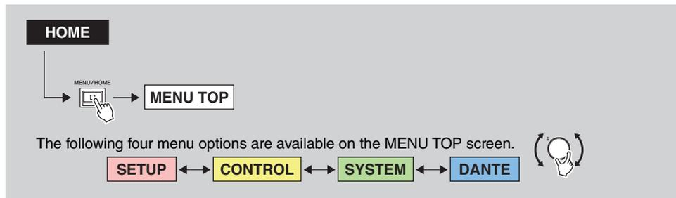
While the home screen is displayed, press the [MENU/HOME] key to display the MENU TOP screen. Turn the encoder with switch to select a menu option, and then press it to confirm.
