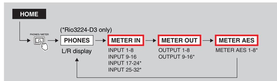
While the home screen is displayed, press the [PHONES/METER] key to display the PHONES screen. Press the [PHONES/METER] key repeatedly to switch screens.
