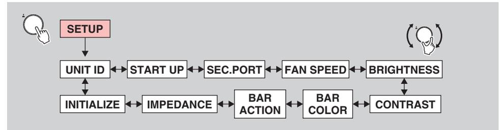
While the SETUP screen is displayed, turn the encoder with switch to select a parameter, and then press it to confirm.
