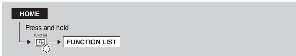
While the home screen is displayed, press and hold the [FUNCTION] key to display the FUNCTION LIST screen.
