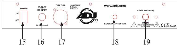
15. POWER SWITCH - Accepts a DC 9V~12V, 300mA minimum, power supply.
