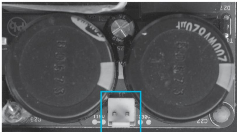
110 VAC operation: it is possible to operate the unit at 110 (115) VAC.
