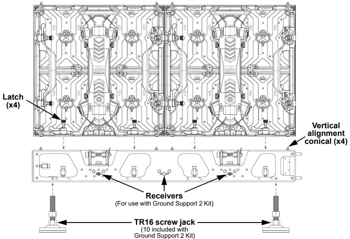
1. Insert alignment conicals into the alignment holes and allow magnets to connect.
