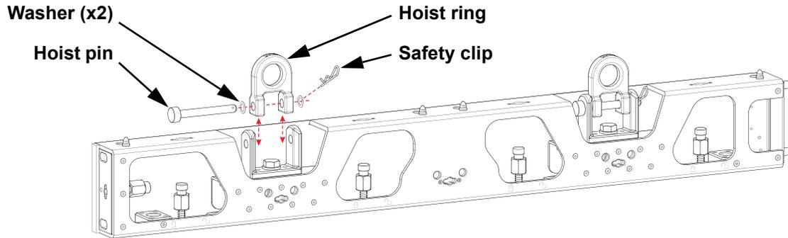
1. Remove the safety clip from the hoist pin.
