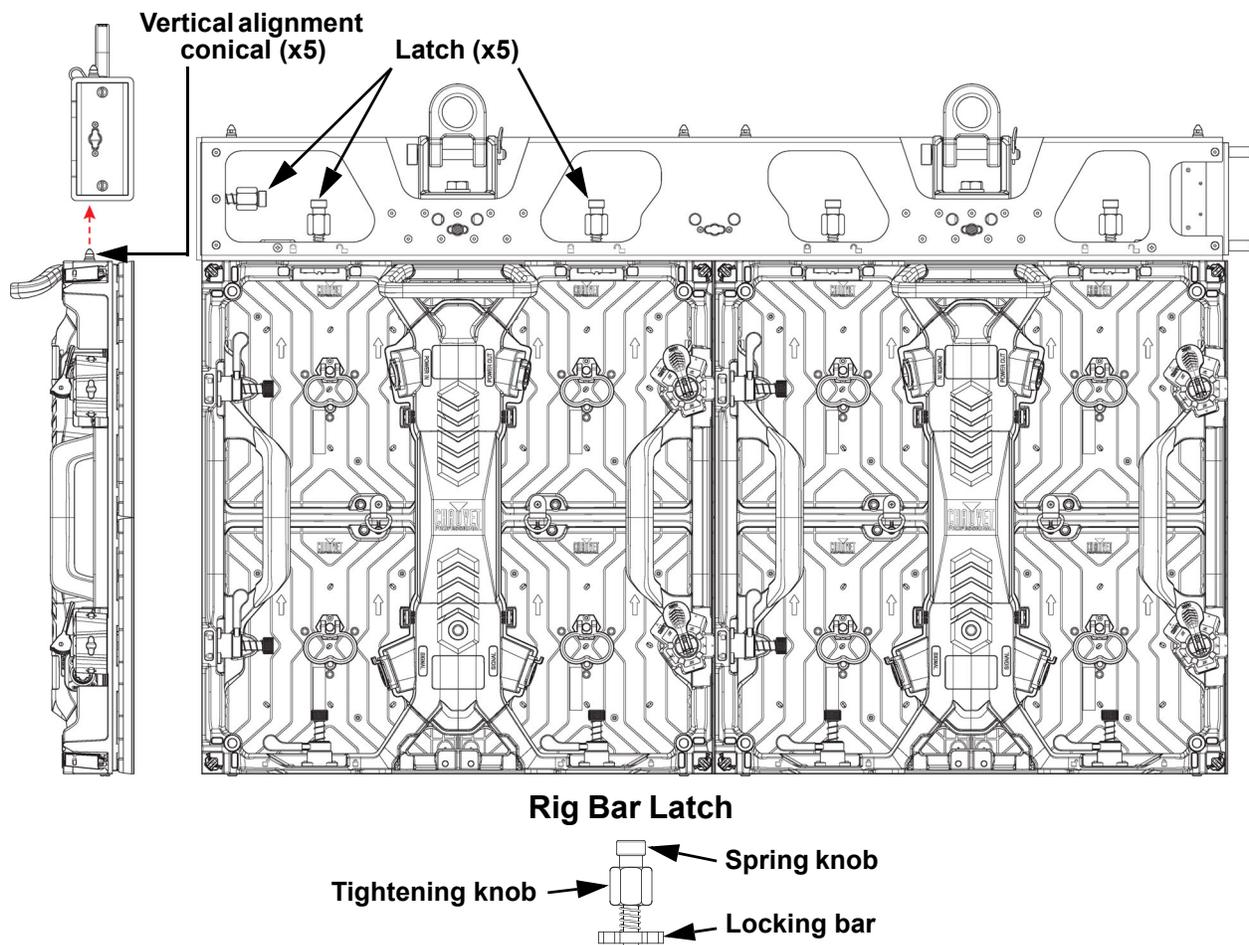
1. Insert alignment conicals into the alignment holes and allow magnets to connect.
