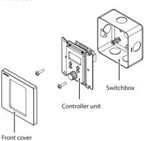
NOTE To remove the front cover, insert a flat head screwdriver, for example into the cutouts at its top and the bottom to pry it off. Be careful not to damage the front cover when doing this.
