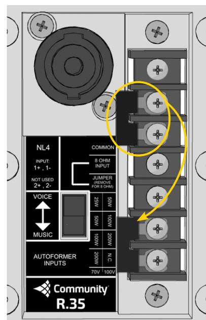
Must remove jumper, or move it to the bottom terminals, for 8Ω operation (see yellow arrow)
