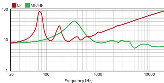
Min Impedance: (LF) 9.3 ohms @ 250Hz, (MF/HF) 5.6 ohms @ 5000 Hz
