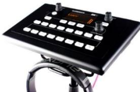
If you are using the Allen & Heath ME personal mixing system then connect it to the dSNAKE, EXPANDER or MONITOR (AR2412 only) port. ME-1 mixers can be daisy chained or you can connect individually via the Allen & Heath ME-U PoE hub.
