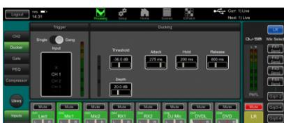
**Channel Ducker** – You can insert a ducker into input channels or groups. This lets you use any signal to automatically duck (attenuate) other channels when active. For example, to use a paging mic as a trigger to duck a background music channel when in use.
