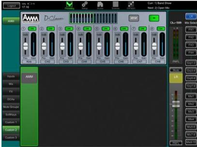
**Automatic Mic Mixing (AMM)** – This is very useful for speech applications such as conferences and seminars involving several microphones around a table. The Qu AMM can automatically take over the level of these mics to improve clarity and reduce the risk of feedback caused by many open microphones.
