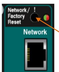
**Qu network address** - The mixer must have a TCP/IP (network) address compatible with the router. The Qu default is DHCP enabled which means that the router will automatically allocate a compatible address to the mixer when connected. If the mixer address has been changed and the Qu-Pad app does not connect then you can reset it to this default:
