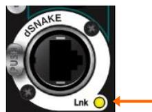
If you are using an AudioRack or the ME personal mixing system then the yellow dSNAKE Lnk indicator will flash steadily once connection is established.
