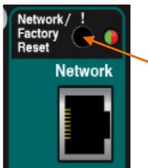
A power-up reset is available if you need to fully reset the Qu mixer settings and its memories. This could be done to clear the system out before sending the mixer to a client, or if you suspect a system problem.
