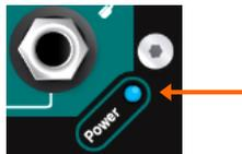
**Switching the mixer on** – Qu-SB does not have a power switch. Plug the provided IEC mains cord into the mixer AC MAINS IN socket. Turn power on at the mains inlet if it is not on already. The mixer takes just a few seconds to boot up. It restores its previous settings and audio.
