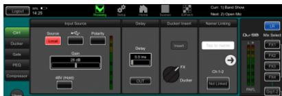
**Choose the channels sources** – You can choose one of 3 sources for each mono and stereo channel – Local socket (rear panel), dSNAKE socket (remote IO), or USB (playback). The reset default is the Local input sources.
