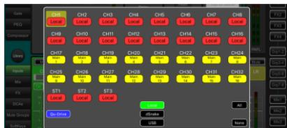
To change channel sources use the **Processing** screen Preamp tab Source button. If you are using dSNAKE you can patch any remote socket to any channel. If you are using USB select either Qu-Drive or USB B as the global source.
