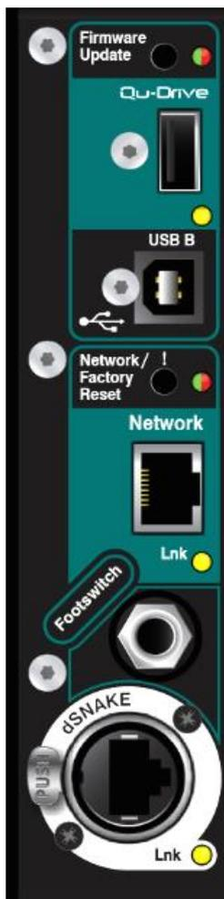
**1 Network Port** – Qu-SB is controlled using an iPad running the Allen & Heath Qu-Pad app. Connect a wireless router (wireless access point) to this port to set up a Wi-Fi network for the iPad to connect to the mixer. This is described in more detail later in this guide.
