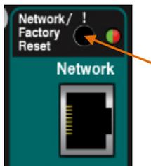
There are two reset functions available using the Qu-SB recessed panel switch above the Network socket.
