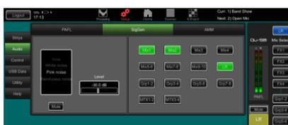
**Signal Generator** – The Qu mixer has a built-in signal generator. Pink noise is an excellent source for testing speakers. It generates equal energy per octave across all frequencies and can be used to check that all speaker drivers are working and to listen for phasing and polarity issues.
