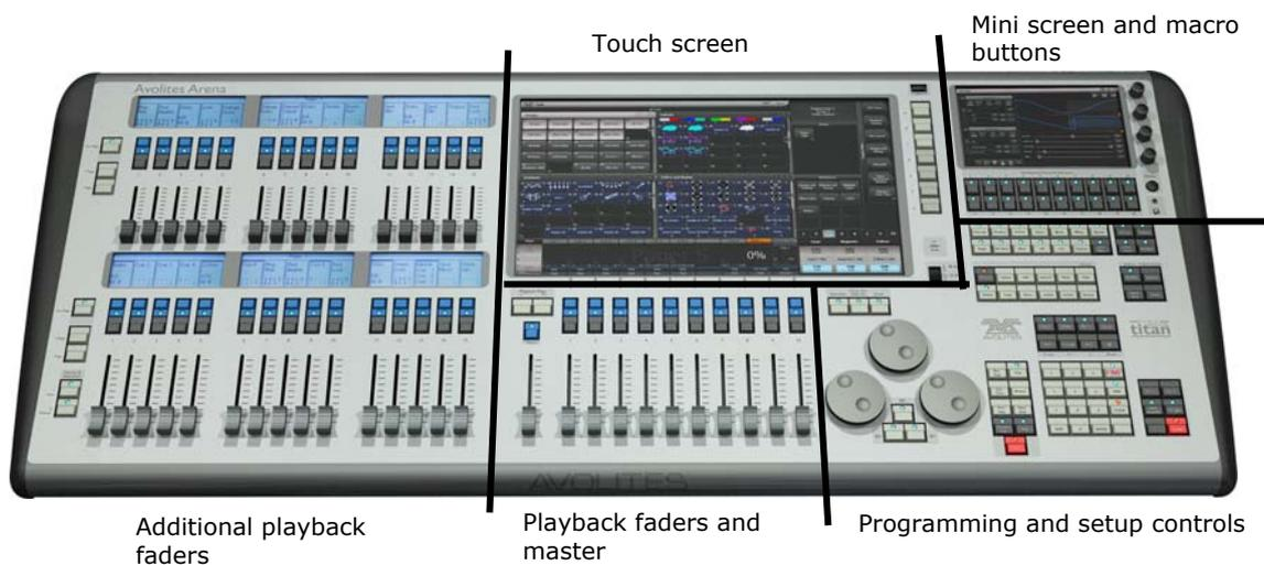
The **Touch screen** contains fixture, palette and group select buttons. It also shows legends for the playback faders and shows the current menu page and softkey buttons on the top right of the screen.
