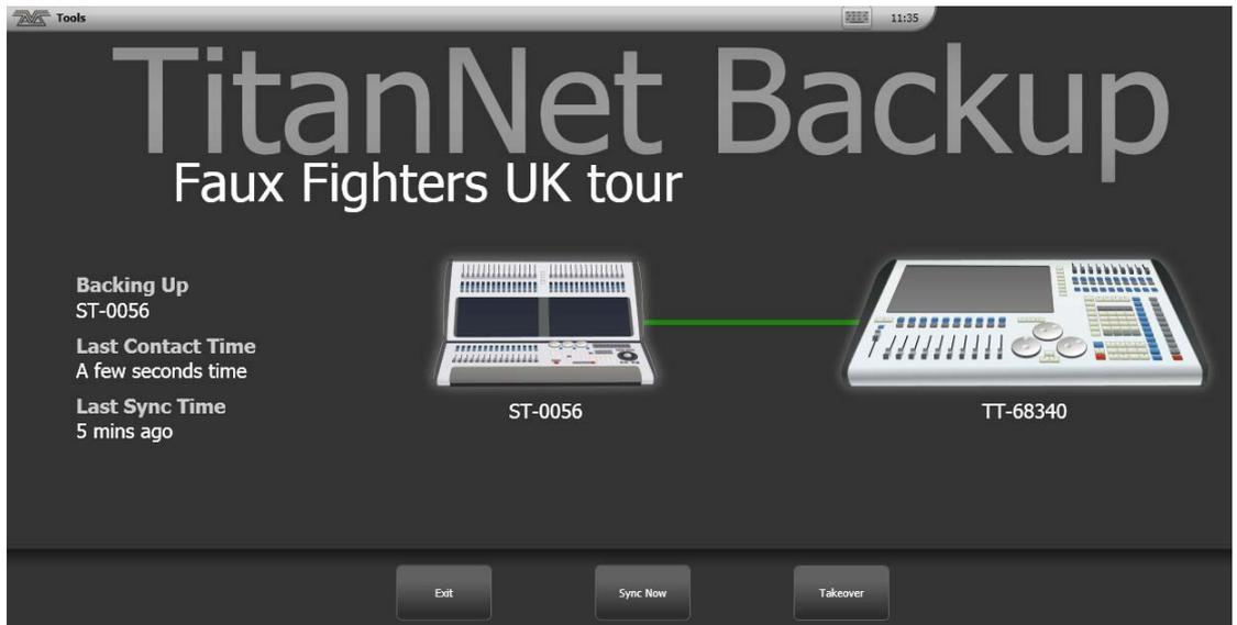
A green line between consoles represents a good connection. If a red line is shown there is a problem with the network connection. A blue line will appear during sync operations.
