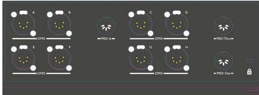
All the connections required for the console are found on the back panel. There are 8 DMX outputs on 5-pin XLR, MIDI in/out/thru on 5-pin DIN, two desk lamp sockets, four Ethernet sockets from the internal Ethernet switch, an Opticon Duo optical terminal for fibre network, a DVI connector for external monitor, three USB sockets, SMPTE input, audio input on 1/4 inch jack and remote trigger terminal on 1/4 inch jack.
