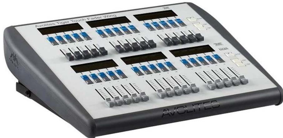
The Tiger Touch Wing connects by USB to the main console. It also needs a mains power connection. The Wing has a built in USB hub to provide 2 further USB sockets for a keyboard etc.
