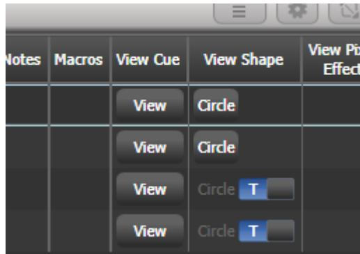
In the following cues where shapes are tracking, an option switch is shown for each active shape.
