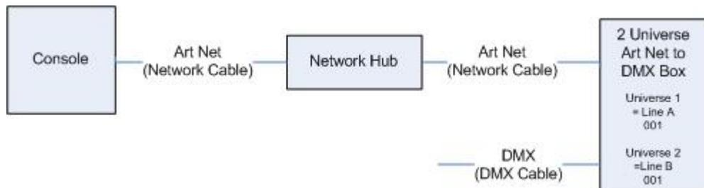
Using standard RJ45 ethernet cables, attach the devices together.
