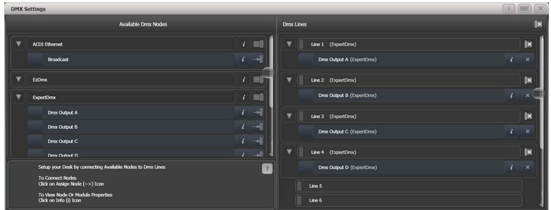
You can individually assign Nodes to Lines using the arrow button, or assign all Nodes of the same type using the group assign button. For example, to assign each XLR output socket on the back of the console to a DMX line, you would click on the Group Assign button of the ExpertDMX nodes.
