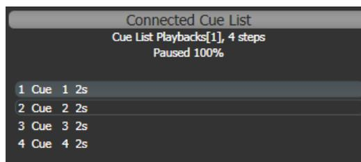
Also the display relating to the playback fader shows information about the cue list, including the current and next cue, fade progress of the current cue, and fade in/out times.
