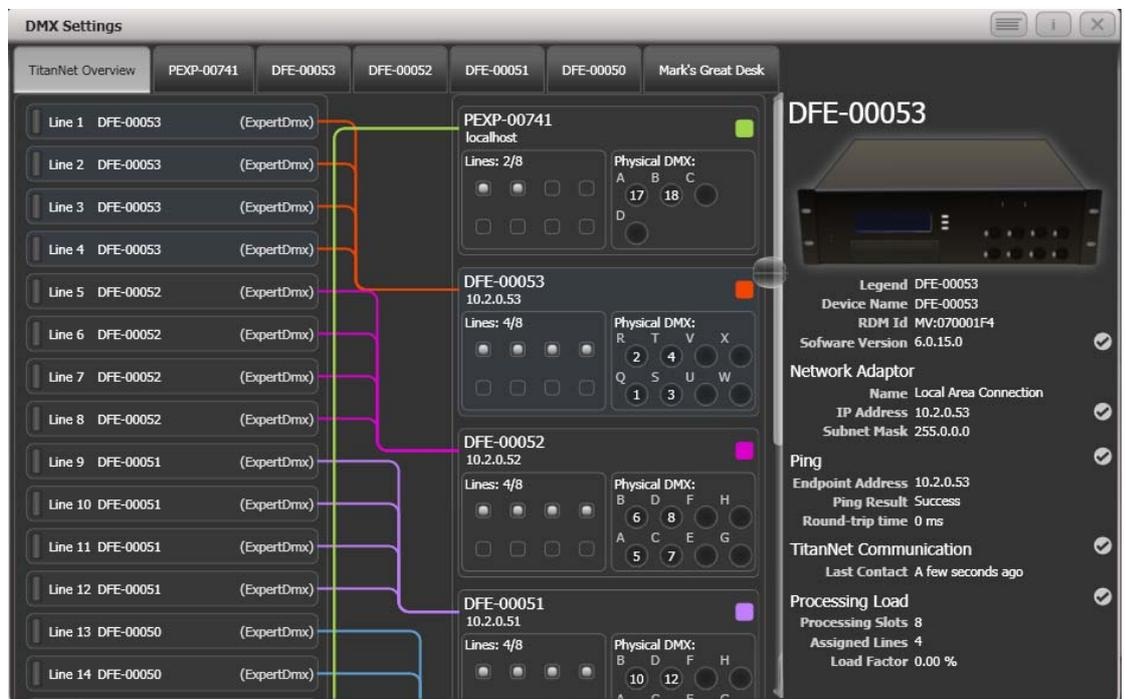
The left side of the screen shows the 64 possible DMX output lines on the console. To the right of this are the processing nodes which are connected, the top one being the console itself. Each node shows how the lines are allocated to the physical outputs on the device. Clicking this area will open the detail tab for the node.
