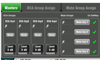
**Name the channels and masters** – Working from your plot sheet, use the mixer **Processing** screens to enter names with up to 6 characters. Touch the name to open the keypad. The Qu-Pad app can also be used to enter names.
