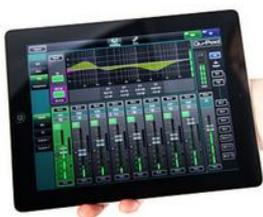
**Qu-Pad** is an engineer's mixing tool giving you the freedom to walk the room or stage and control the sound where it is needed. Qu-Pad follows the User Profiles and Permissions as set in the Qu mixer.
