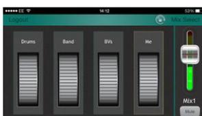
**Qu-You** provides personal monitor mix control for musicians on stage. The engineer can still keep an eye on and control each mix at the Qu mixer at any time. A password for Qu-You users can be set at the mixer.
