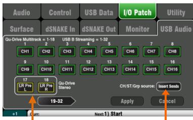
**Qu-Drive recording direct to USB drive** – You can record [stereo](#) or [18-track multitrack](#) direct to a USB storage device plugged into the front panel Qu-Drive port.
