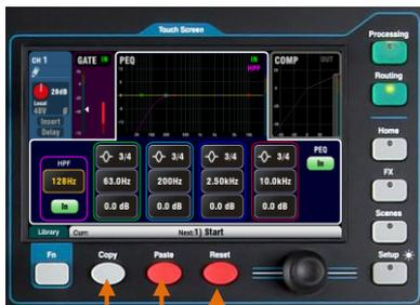
**Copy / Paste / Reset** – These keys provide a powerful tool for quickly setting up your processing. They work in a similar way. Press and hold the key down. While holding, press or touch another item to perform the action:
