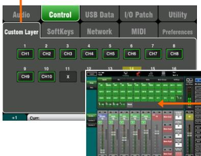
**Assign the Custom Layer** – A third fader strip layer can be user assigned for any combination of channel, FX, mix, DCA and MIDI select. This can give you quick access to just the channels you are using for your show. Assign these using the **Setup / Control / Custom Layer** screen. Use the **Fn** key as a '+1' increment to let you quickly step through a range of assignments.
