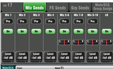
**Routing screen** – This screen lets you work with the sends from one channel to all the mixes, or access global settings and routing options for the mixes. To work with the sends from all channels to one mix use the **Mix** keys.
