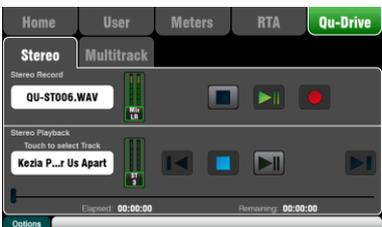
**Patch the sources to record** using the **Setup / I/O Patch / USB Audio** screen. Use the rotary to spin through available sources to each of the 18 tracks. Press the **Fn** key '+1' to increment quickly through the tracks. Choose channel sources to be from Insert Sends or Direct Out.
