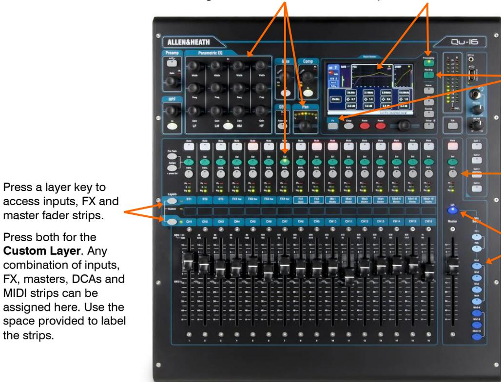
Press a layer key to access inputs, FX and master fader strips.
