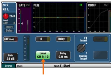
Start by using the **Processing** screen Preamp page **Linking** button to link parameters for any odd/even stereo pairs of channels you may need. For example, stereo keyboards or backing tracks. Adjusting **Pan** on one channel will set the width for the pair.
