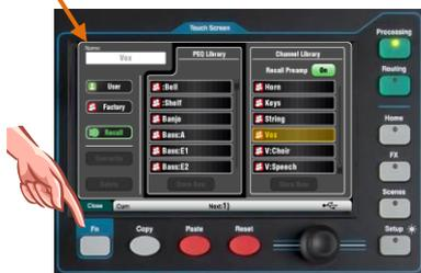
**Channel Library** – This preset recalls all processing (Gate, PEQ, Comp, Delay) for the input channel. Turn on 'Recall Preamp' if you want this to also include the preamp settings (Gain, Pad, 48V, Polarity). Channel libraries do not include the linking or ducker settings.
