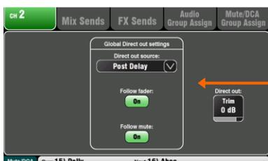
**Patching to the optional ME-1 personal monitor system** - Go to the **Setup / I/O Patch / Monitor** screen to patch Qu outputs to the 40 ME-1 sends. It is typical to send the input channel direct outputs. Recommended direct out setting is post delay, pre fader, post mute.
