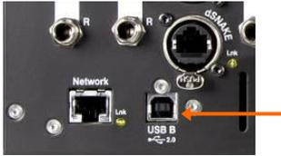
**USB B Streaming** – Connect an Apple® Mac or Windows® PC computer to the rear panel USB B port to stream up to 32 channels of audio in both directions and send MIDI messages.
