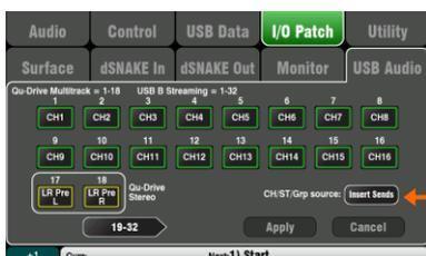
**Patch the USB outputs** – Use the **Setup / I/O Patch / USB Audio** screen to patch any of the Qu outputs to the Qu-Drive multitrack and rear panel **USB B** streaming port. These share the same patch. USB streaming uses all 32 outputs (24 on Qu-16). Qu-Drive recording is fed from the first 18 outputs. Qu-Drive stereo recording is fed from outputs 17-18.
