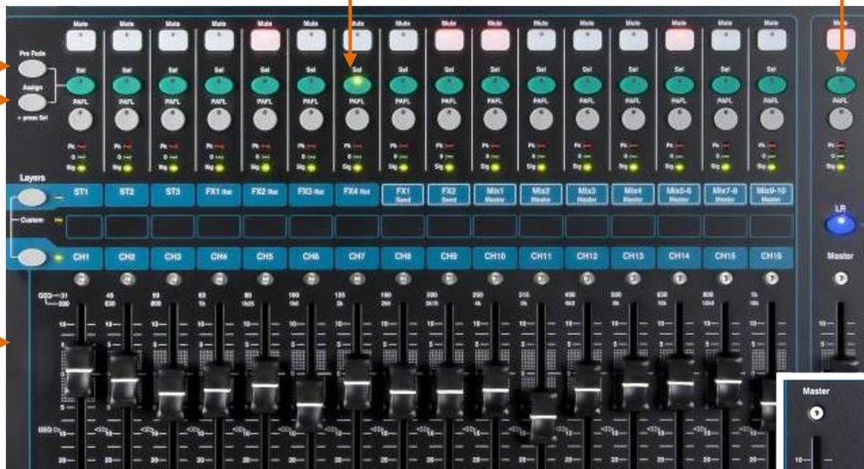
Press a **Group Mix** key to assign its routing and access its master fader and processing. The channel faders remain active. Groups are not available on the Qu-16.
