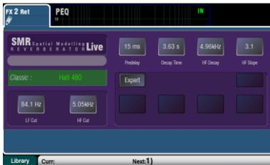
**FX Parameters** – Select an FX Send or Return channel and open the **Processing** screen to view and work with its effects parameters. Touch 'Expert' if you wish to experiment with many more of its advanced parameters. Use the **Fn** key to open the Library page to change the FX type and store or recall presets.
