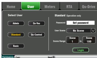
Qu features several functions that protect the system from unauthorised mixer or app access, and restrict how much control is given to certain operators. For example, to prevent a regular event operator from changing the configuration, or to limit non-technical bar staff to simple control of just the background music and paging.
