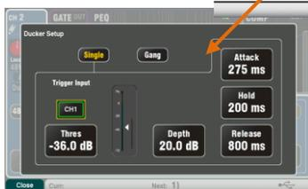
**Channel Ducker** – You can insert a ducker into input channels or groups. This lets you use any Qu signal to automatically duck (attenuate) other channels when active. For example, use a paging mic as a trigger to duck the background music channel. Adjust how fast it ducks and recovers.
