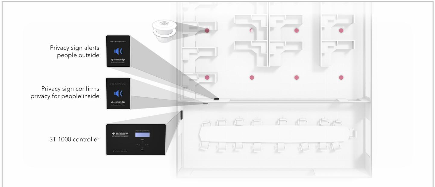
**Example:** Conference room with two exposed walls and an open area extending away from the area in one direction. One row of emitters in side cubicle area.
