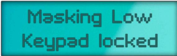
Input A will be ON regardless of masking level or contact closure setting. (Meaning paging – if used – would work even if masking is off).
