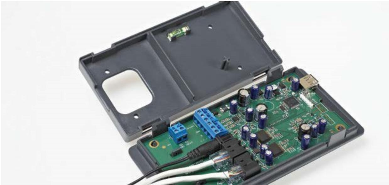
All connections are made to the control module and then the module 'snaps' into place on the wall mount.
