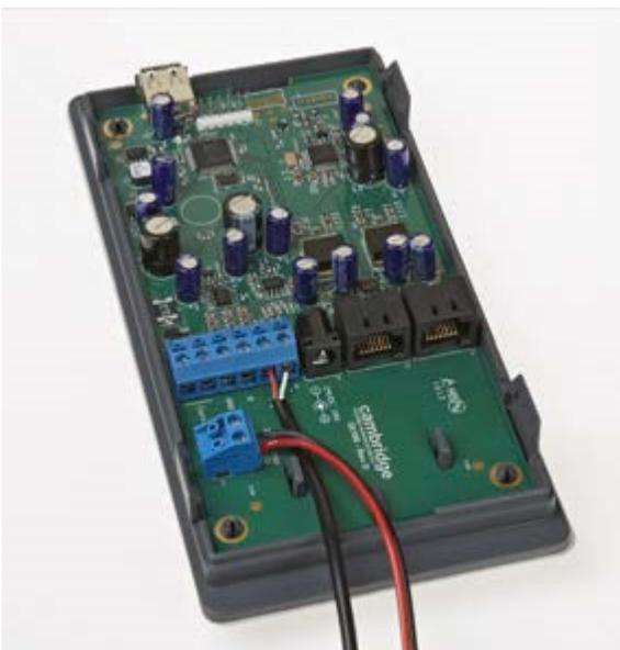
Alternatively, power can be supplied to the fixed block connector, which allows for stripped and tinned wires for added flexibility and convenience.
