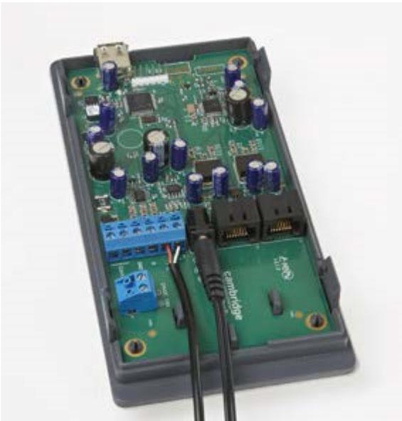
The controller comes standard with a 24 V wall plug power supply. This supply features a wall plug and a fixed barrel connector.
