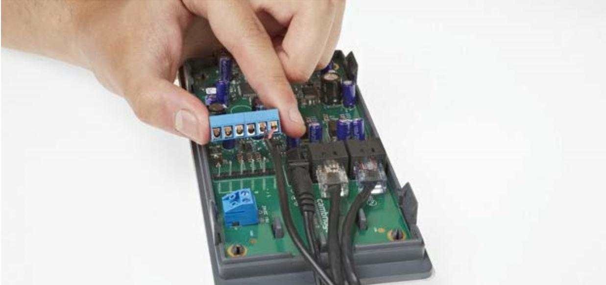
**NOTE:** The fixed terminal block can be removed for ease of connecting.
