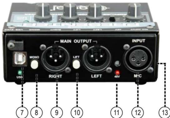
7. **USB:** Provides power for the Presenter and allows playback of high quality audio from a laptop.
