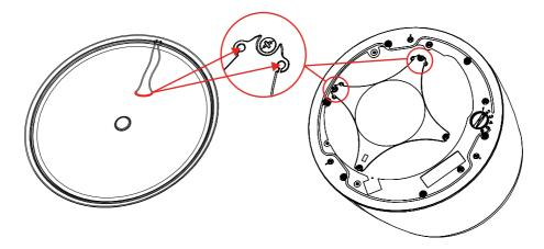
3. Hang the speaker by connecting the carabiner of the suspension cable (included) in the hole A of the bracket.
